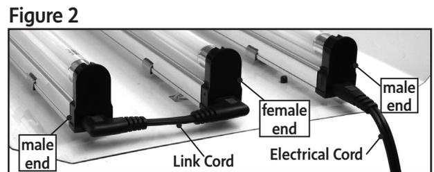
**Step 3.** Plug the Electrical Cord into the male end on an outside Ballast. On the same end of the Light Fixture, connect the other two Ballasts together by plugging in a Link Cord, as shown in Figure 2. Snap it firmly into place. **Important:** The Link Cord is specifically molded to fit only one way on the end of each Ballast. If it does not fit, make sure the Ballasts are positioned with alternate male and female sockets at each end of the Light fixture.
