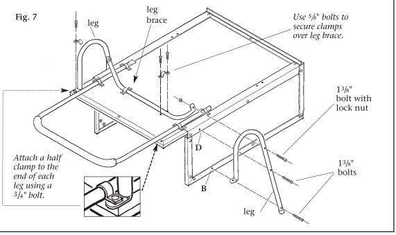
clamp. Fully tighten all bolts and nuts on the legs, leg brace, and handle.
