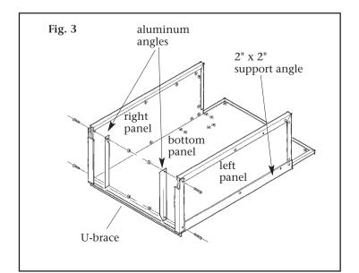
bolts into each side (four total) from the outside. Using a wrench and Phillips screwdriver, firmly tighten the bolts on the inside with a lock nut (Fig. 3). The Ubrace and Aluminum Angles provide a channel for the Front Panel to slide up and down.
