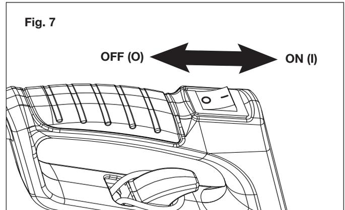
3. To stop the unit, press down (O) on the ON/OFF switch, as indicated (Fig. 7).
