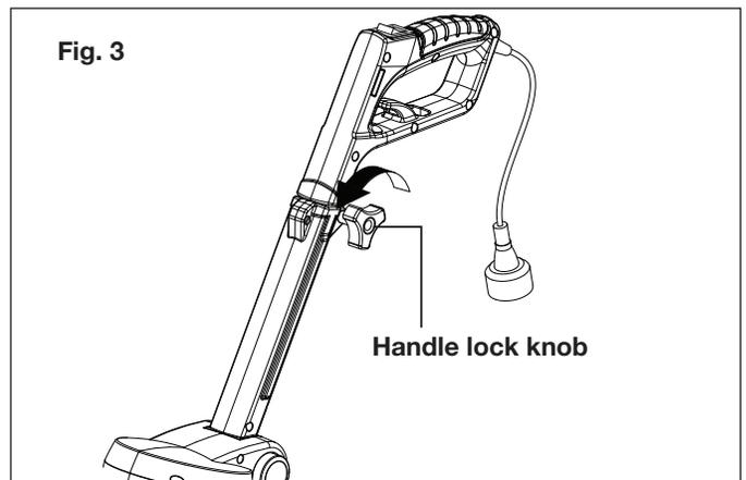
3. With the handle raised in the operating position, extend to the desired height. Turn the handle lock knob clockwise to lock the handle (Fig. 4).
