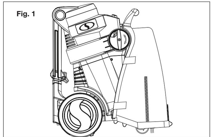
1. Press the handle angle adjustment button, at the same time, rotate the handle up until it locks into the working position (Fig. 2).
