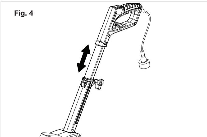
**⚠ WARNING!** To avoid personal injury, make sure the handle is locked securely after adjusting the length.
