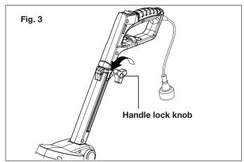
**3.** With the handle raised in the operating position, extend to the desired height. Turn the handle lock knob clockwise to lock the handle (Fig. 4).
